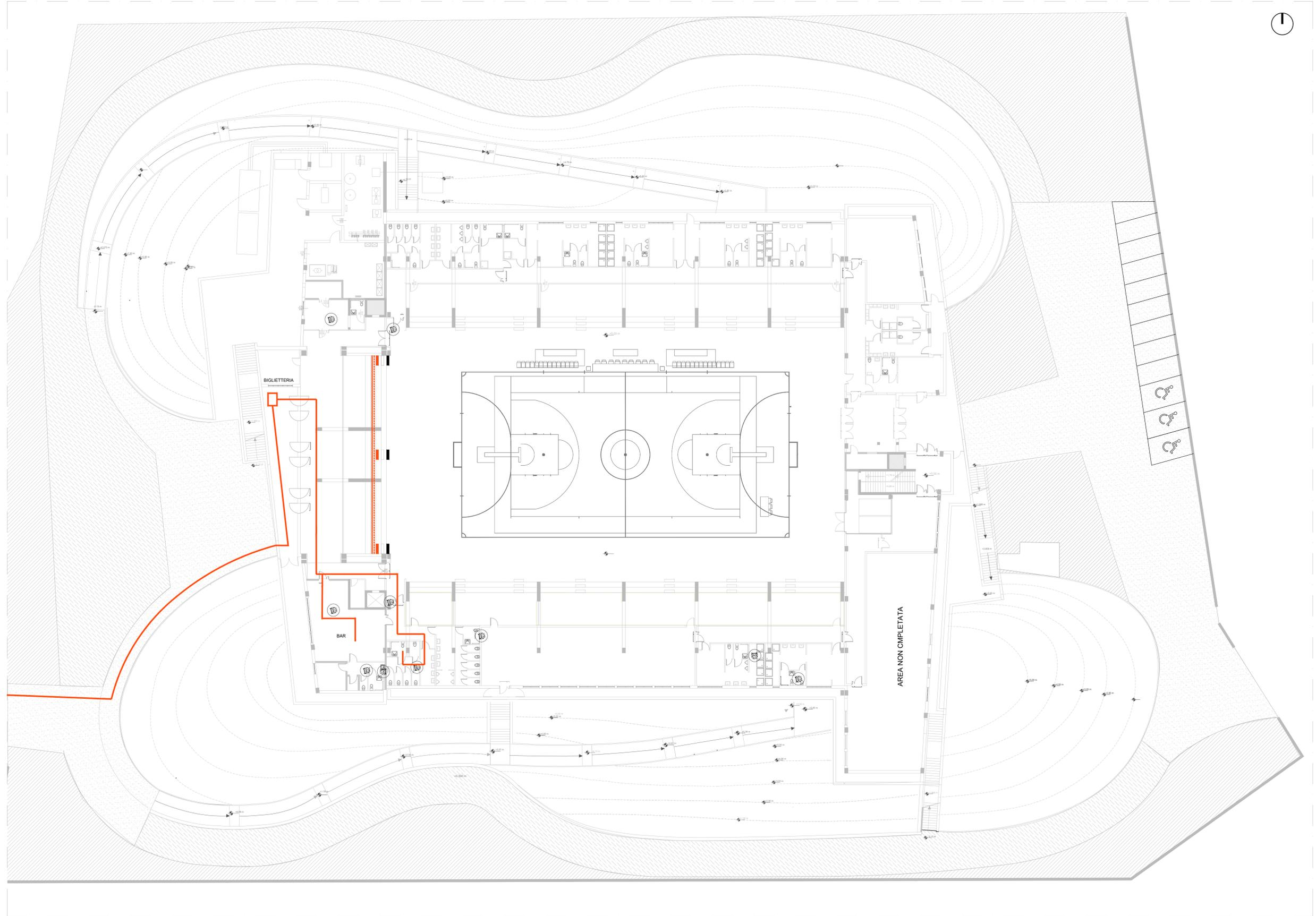
PIANTA PIANO TERRA ACCESSIBILITA' PORTATORI DI HANDICAP MOTORI E VISIVI\_ SCALA 1:200
